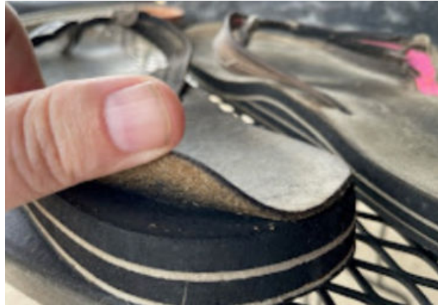
Figure 2 Delamination of Mr. Sher's sandal.
